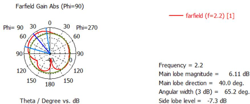
Figure 4:  $\epsilon_r = 2.2$  Multi Substrate with Rect. Patch and H=1.6 Mm and Frequency=2.2 GHz, Beam Width=65.2
