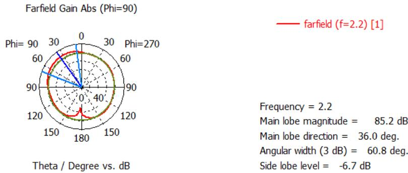
Figure 2:  $\epsilon_r = 2.2$  Single Substrate with Rect. Patch and H=1.6 Mm and Frequency=2.2 GHz, Beam Width=60.8
