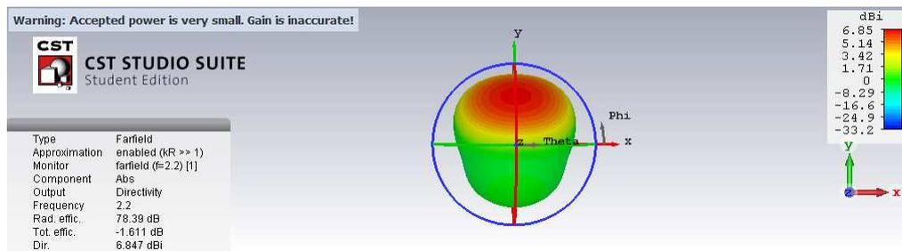
Figure 3:  $\epsilon_r = 2.2$  Single Substrate with Rect. Patch and H=1.6 Mm and Frequency=2.2 GHz, Directivity = 6.847
