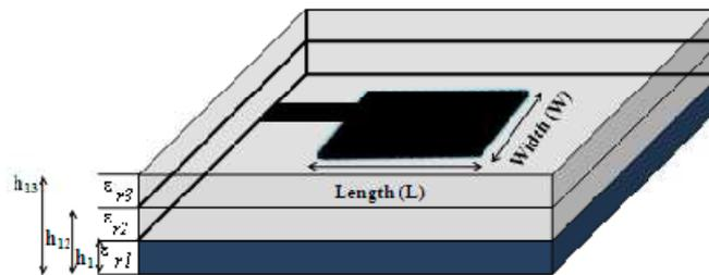
**Figure 1: Multi Layer Microstrip Patch Antenna**
