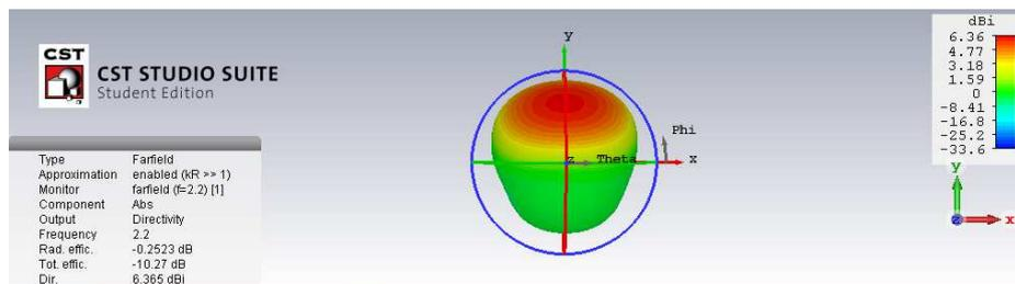
Figure 5:  $\epsilon_r = 2.2$  Single Substrate with Rect. Patch and H=1.6 Mm and Frequency=2.2 GHz, Directivity = 6.365
